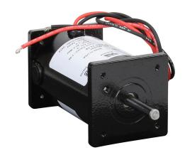
IronHorse MTPM DC permanent magnet motor, SCR-PWM rated, 1/31hp, 90 VDC, 1797rpm, TENV, small frame, rolled steel, flange mount.
