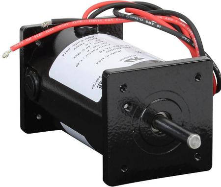
IronHorse MTPM DC permanent magnet motor, SCR-PWM rated, 1/31hp, 90 VDC, 1797rpm, TENV, small frame, rolled steel, flange mount.
