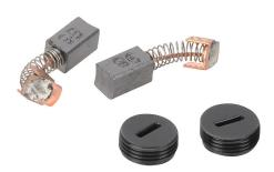
IronHorse DC motor brushes, replacement. Package of 2. For use with IronHorse 1/10hp or smaller 90 VDC or 180 VDC MTPM, MTGR, and MTGP series permanent magnet DC motors and gearmotors. (2) brush caps included.
