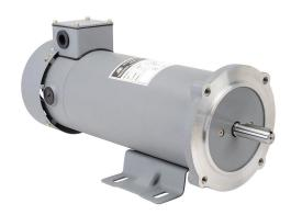
IronHorse MTPM DC permanent magnet motor, SCR-PWM rated, 1-1/2hp, 180 VDC, 1800rpm, TEFC, 56C frame, rolled steel, C-face/removable rigid base mount. Replacement brushes included.
