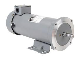
IronHorse MTPM DC permanent magnet motor, SCR-PWM rated, 1-1/2hp, 90 VDC, 1800rpm, TEFC, 56C frame, rolled steel, C-face/removable rigid base mount. Replacement brushes included.
