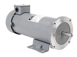
IronHorse MTPM DC permanent magnet motor, SCR-PWM rated, 1-1/2hp, 90 VDC, 1800rpm, TEFC, NEMA 56C frame, rolled steel, C-face/removable rigid base mount. Replacement brushes included.
