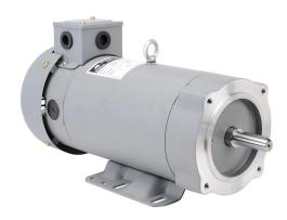
IronHorse MTPM DC permanent magnet motor, SCR-PWM rated, 2hp, 180 VDC, 1800rpm, TEFC, NEMA 56C frame, rolled steel, C-face/removable rigid base mount. Replacement brushes included.
