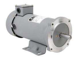
IronHorse MTPM DC permanent magnet motor, SCR-PWM rated, 1hp, 180 VDC, 1800rpm, TEFC, NEMA 56C frame, rolled steel, C-face/removable rigid base mount. Replacement brushes included.
