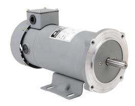
IronHorse MTPM DC permanent magnet motor, SCR-PWM rated, 1hp, 90 VDC, 1800rpm, TEFC, NEMA 56C frame, rolled steel, C-face/removable rigid base mount. Replacement brushes included.
