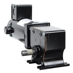
IronHorse right angle single shaft DC gear motor, 1/5hp, 24 VDC, 75rpm, 137 lb-in full load torque, 8.72 FLA, 23:1 ratio, 5/8in shaft diameter.
