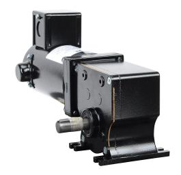
IronHorse right angle single shaft DC gear motor, 1/5hp, 24 VDC, 75rpm, 137 lb-in full load torque, 8.72 FLA, 23:1 ratio, 5/8in shaft diameter.
