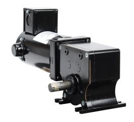
IronHorse right angle single shaft DC gear motor, 1/7hp, 90 VDC, 178rpm, 44 lb-in full load torque, 1.64 FLA, 10:1 ratio, 5/8in shaft diameter.
