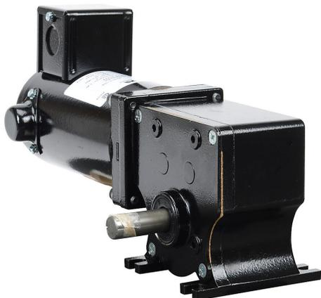
IronHorse right angle single shaft DC gear motor, 1/7hp, 90 VDC, 178rpm, 44 lb-in full load torque, 1.64 FLA, 10:1 ratio, 5/8in shaft diameter.
