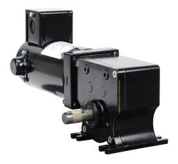
IronHorse right angle single shaft DC gear motor, 1/7hp, 90 VDC, 77rpm, 97 lb-in full load torque, 1.65 FLA, 23:1 ratio, 5/8in shaft diameter.
