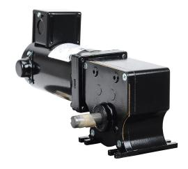
IronHorse right angle single shaft DC gear motor, 1/7hp, 90 VDC, 22rpm, 280 lb-in full load torque, 1.41 FLA, 82:1 ratio, 5/8in shaft diameter.
