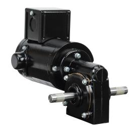
IronHorse right angle dual shaft DC gear motor, 1/15hp, 12 VDC, 177rpm, 18 lb-in full load torque, 6.78 FLA, 9.75:1 ratio, 1/2in shaft diameter.
