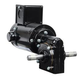
IronHorse right angle dual shaft DC gear motor, 1/15hp, 12 VDC, 84rpm, 34 lb-in full load torque, 6.78 FLA, 20.5:1 ratio, 1/2in shaft diameter.
