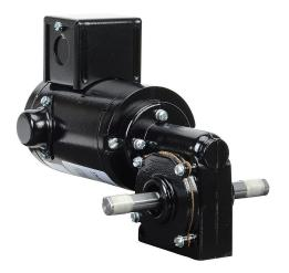
IronHorse right angle dual shaft DC gear motor, 1/15hp, 12 VDC, 36rpm, 50 lb-in full load torque, 5.69 FLA, 50:1 ratio, 1/2in shaft diameter.
