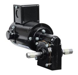
IronHorse right angle dual shaft DC gear motor, 1/19hp, 90 VDC, 197rpm, 12 lb-in full load torque, 0.68 FLA, 9.75:1 ratio, 1/2in shaft diameter.
