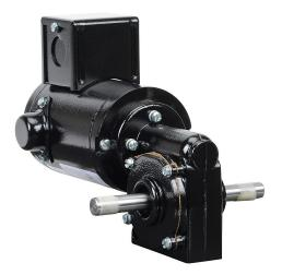
IronHorse right angle dual shaft DC gear motor, 1/19hp, 90 VDC, 132rpm, 17 lb-in full load torque, 0.67 FLA, 14.5:1 ratio, 1/2in shaft diameter.
