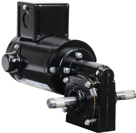
IronHorse right angle dual shaft DC gear motor, 1/19hp, 90 VDC, 53rpm, 33 lb-in full load torque, 0.68 FLA, 36:1 ratio, 1/2in shaft diameter.
