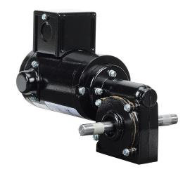
IronHorse right angle dual shaft DC gear motor, 1/19hp, 90 VDC, 38rpm, 42 lb-in full load torque, 0.68 FLA, 50:1 ratio, 1/2in shaft diameter.
