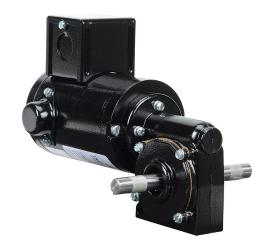
IronHorse right angle dual shaft DC gear motor, 1/19hp, 90 VDC, 38rpm, 42 lb-in full load torque, 0.68 FLA, 50:1 ratio, 1/2in shaft diameter.
