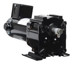
IronHorse parallel shaft DC gear motor, 1/5hp, 12 VDC, 154rpm, 61 lb-in full load torque, 15.6 FLA, 11:1 ratio, 5/8in shaft diameter.
