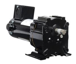
IronHorse parallel shaft DC gear motor, 1/5hp, 12 VDC, 84rpm, 112 lb-in full load torque, 15.7 FLA, 20:1 ratio, 5/8in shaft diameter.
