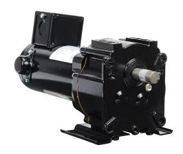
IronHorse parallel shaft DC gear motor, 1/5hp, 12 VDC, 84rpm, 112 lb-in full load torque, 15.7 FLA, 20:1 ratio, 5/8in shaft diameter.
