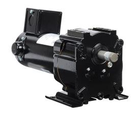
IronHorse parallel shaft DC gear motor, 1/5hp, 12 VDC, 56rpm, 168 lb-in full load torque, 15.7 FLA, 30:1 ratio, 5/8in shaft diameter.
