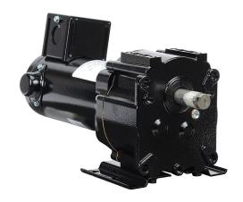
IronHorse parallel shaft DC gear motor, 1/5hp, 12 VDC, 37rpm, 245 lb-in full load torque, 15.8 FLA, 46:1 ratio, 5/8in shaft diameter.
