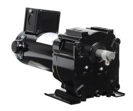
IronHorse parallel shaft DC gear motor, 1/5hp, 12 VDC, 26rpm, 280 lb-in full load torque, 12.6 FLA, 69:1 ratio, 5/8in shaft diameter.
