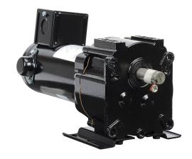
IronHorse parallel shaft DC gear motor, 1/7hp, 90 VDC, 165rpm, 47 lb-in full load torque, 1.57 FLA, 11:1 ratio, 5/8in shaft diameter.
