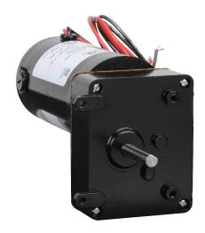
IronHorse parallel shaft DC gear motor, 1/17hp, 90 VDC, 114rpm, 26 lb-in full load torque, 0.61 FLA, 26:1 ratio, 5/16in shaft diameter.
