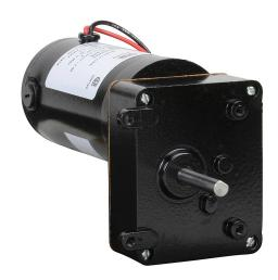
IronHorse parallel shaft DC gear motor, 1/17hp, 90 VDC, 55rpm, 45 lb-in full load torque, 0.54 FLA, 55:1 ratio, 5/16in shaft diameter.
