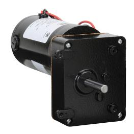
IronHorse parallel shaft DC gear motor, 1/17hp, 90 VDC, 12rpm, 50 lb-in full load torque, 0.23 FLA, 269:1 ratio, 5/16in shaft diameter.
