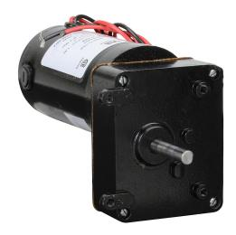
IronHorse parallel shaft DC gear motor, 1/17hp, 90 VDC, 8.4rpm, 50 lb-in full load torque, 0.19 FLA, 386:1 ratio, 5/16in shaft diameter.
