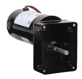
IronHorse parallel shaft DC gear motor, 1/16hp, 12 VDC, 97rpm, 36 lb-in full load torque, 5.68 FLA, 26:1 ratio, 5/16in shaft diameter.
