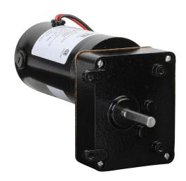
IronHorse parallel shaft DC gear motor, 1/16hp, 12 VDC, 97rpm, 36 lb-in full load torque, 5.68 FLA, 26:1 ratio, 5/16in shaft diameter.
