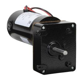
IronHorse parallel shaft DC gear motor, 1/16hp, 12 VDC, 50rpm, 45 lb-in full load torque, 3.88 FLA, 55:1 ratio, 5/16in shaft diameter.
