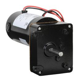
IronHorse parallel shaft DC gear motor, 1/16hp, 12 VDC, 34rpm, 45 lb-in full load torque, 2.86 FLA, 83:1 ratio, 5/16in shaft diameter.
