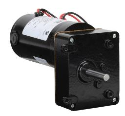
IronHorse parallel shaft DC gear motor, 1/16hp, 12 VDC, 7.9rpm, 50 lb-in full load torque, 1.39 FLA, 386:1 ratio, 5/16in shaft diameter.
