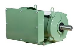
IronHorse MTF2 standard efficiency AC induction motor, general purpose and farm duty, 7-1/2hp, 1-phase, 208-230 VAC, 1800rpm, TEFC, 215T frame, rolled steel, rigid base mount.
