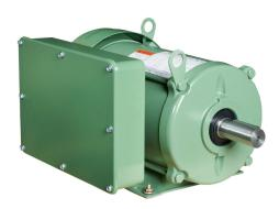
IronHorse MTF2 standard efficiency AC induction motor, general purpose and farm duty, 10hp, 1-phase, 208-230 VAC, 1800rpm, TEFC, 215T frame, rolled steel, rigid base mount.
