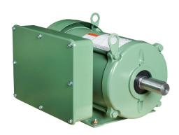
IronHorse MTF2 standard efficiency AC induction motor, general purpose and farm duty, 10hp, 1-phase, 208-230 VAC, 1800rpm, TEFC, NEMA 215T frame, rolled steel, rigid base mount.
