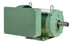
IronHorse MTF2 standard efficiency AC induction motor, general purpose and farm duty, 5hp, 1-phase, 208-230 VAC, 1800rpm, TEFC, NEMA 184T frame, rolled steel, rigid base mount.
