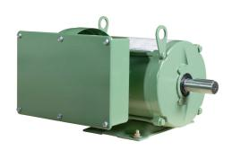
IronHorse MTF2 standard efficiency AC induction motor, general purpose and farm duty, 3hp, 1-phase, 208-230 VAC, 1800rpm, TEFC, NEMA 184T frame, rolled steel, rigid base mount.
