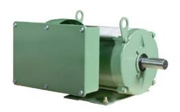
IronHorse MTF2 standard efficiency AC induction motor, general purpose and farm duty, 3hp, 1-phase, 208-230 VAC, 1800rpm, TEFC, 184T frame, rolled steel, rigid base mount.
