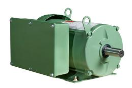
IronHorse MTF2 standard efficiency AC induction motor, general purpose and farm duty, 2hp, 1-phase, 208-230 VAC, 1800rpm, TEFC, NEMA 182T frame, rolled steel, rigid base mount.
