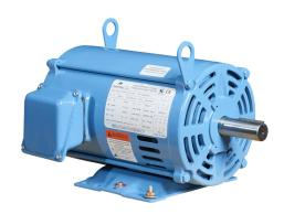
IronHorse MTDP high efficiency AC induction motor, general purpose and inverter rated, 7-1/2hp, 3-phase, 208-230/460 VAC, 3600rpm, ODP, NEMA 184T frame, rolled steel, rigid base mount.
