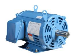
IronHorse MTDP premium efficiency AC induction motor, general purpose and inverter rated, 7-1/2hp, 3-phase, 208-230/460 VAC, 1800rpm, ODP, NEMA 213T frame, rolled steel, rigid base mount.
