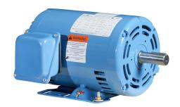
IronHorse MTDP premium efficiency AC induction motor, general purpose and inverter rated, 1-1/2hp, 3-phase, 208-230/460 VAC, 1800rpm, ODP, NEMA 145T frame, rolled steel, rigid base mount.
