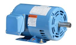
IronHorse MTDP premium efficiency AC induction motor, general purpose and inverter rated, 1-1/2hp, 3-phase, 208-230/460 VAC, 1800rpm, ODP, 145T frame, rolled steel, rigid base mount.
