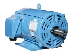
IronHorse MTDP premium efficiency AC induction motor, general purpose and inverter rated, 50hp, 3-phase, 208-230/460 VAC, 1800rpm, ODP, NEMA 326T frame, rolled steel, rigid base mount.
