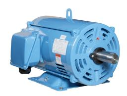
IronHorse MTDP premium efficiency AC induction motor, general purpose and inverter rated, 40hp, 3-phase, 208-230/460 VAC, 1800rpm, ODP, NEMA 324T frame, rolled steel, rigid base mount.
