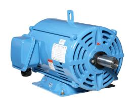
IronHorse MTDP premium efficiency AC induction motor, general purpose and inverter rated, 30hp, 3-phase, 208-230/460 VAC, 1800rpm, ODP, NEMA 286T frame, rolled steel, rigid base mount.
