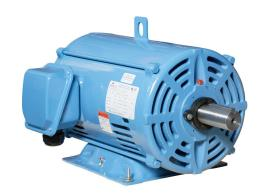
IronHorse MTDP premium efficiency AC induction motor, general purpose and inverter rated, 25hp, 3-phase, 208-230/460 VAC, 1800rpm, ODP, NEMA 284T frame, rolled steel, rigid base mount.
