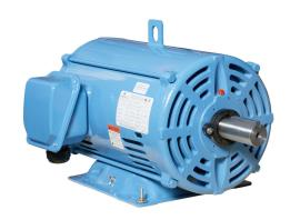
IronHorse MTDP premium efficiency AC induction motor, general purpose and inverter rated, 25hp, 3-phase, 208-230/460 VAC, 1800rpm, ODP, 284T frame, rolled steel, rigid base mount.
