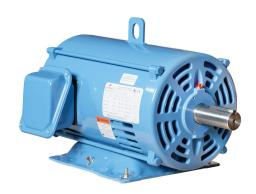
IronHorse MTDP premium efficiency AC induction motor, general purpose and inverter rated, 20hp, 3-phase, 208-230/460 VAC, 1800rpm, ODP, NEMA 256T frame, rolled steel, rigid base mount.
