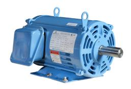
IronHorse MTDP premium efficiency AC induction motor, general purpose and inverter rated, 10hp, 3-phase, 208-230/460 VAC, 1800rpm, ODP, NEMA 215T frame, rolled steel, rigid base mount.
