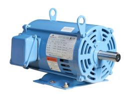
IronHorse MTDP premium efficiency AC induction motor, general purpose and inverter rated, 5hp, 3-phase, 208-230/460 VAC, 3600rpm, ODP, NEMA 182T frame, rolled steel, rigid base mount.
