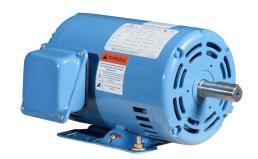
IronHorse MTDP premium efficiency AC induction motor, general purpose and inverter rated, 3hp, 3-phase, 208-230/460 VAC, 3600rpm, ODP, 145T frame, rolled steel, rigid base mount.
