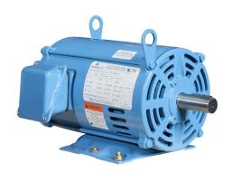
IronHorse MTDP premium efficiency AC induction motor, general purpose and inverter rated, 3hp, 3-phase, 208-230/460 VAC, 1800rpm, ODP, NEMA 182T frame, rolled steel, rigid base mount.
