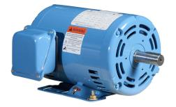
IronHorse MTDP premium efficiency AC induction motor, general purpose and inverter rated, 2hp, 3-phase, 208-230/460 VAC, 1800rpm, ODP, NEMA 145T frame, rolled steel, rigid base mount.
